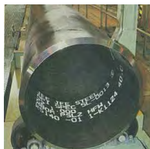
X80-grade pipe with one-inch (25.4mm) thickness made of hot-rolled coil for oil and gas field
